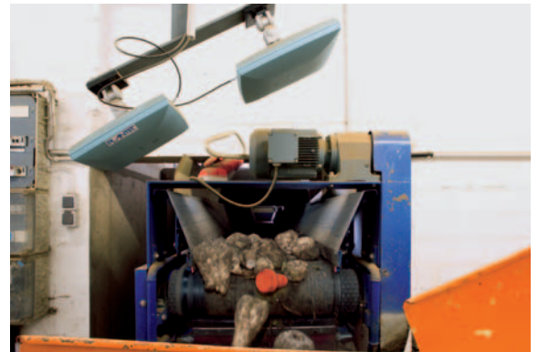
RFID transponders in the data capsules enable the automatic tracing of every batch of sugar beet on its journey through the plant.
