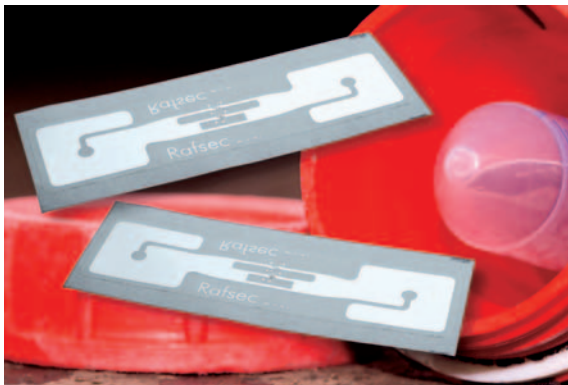
The sturdy data capsule contains an RFID transponder on which the batch's unique identification number is stored.
