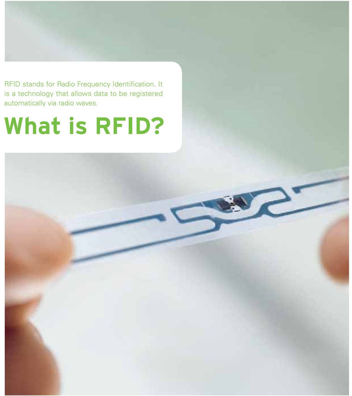
An antenna and a tiny computer chip: this is what an RFID transponder looks like.
